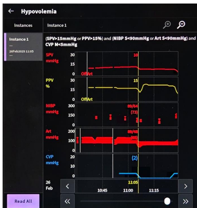
Image: Sample of customized notification implementation for indicators of Hypovolemia combining Pulse or Systolic Pressure Variation (SPV/ PPV), Systolic BP (NIBP / ART) & Central Venous pressure (CPV) measurement thresholds.
