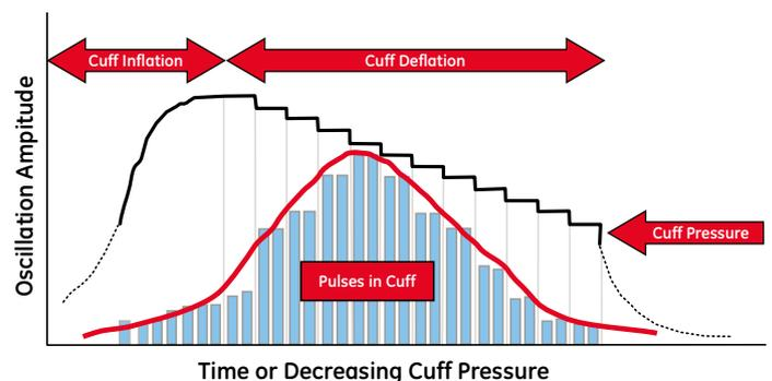
Figure 1. Typical oscillometric envelope used to measure NIBP.
